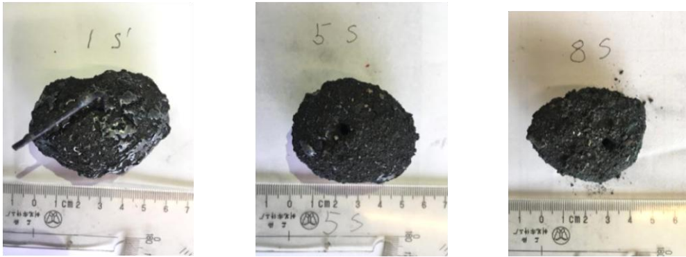
Fig 10 Photo of Mn-C pellet dissolution in molten steel for different time
